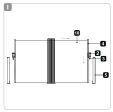
⚠ CAUTION! RISK OF INJURY! Make sure that you hold onto the profile 4 handle 2 tightly. Only let go once the profile 4 is secured into the support post 5 (see fig. J). Because: The more you pull the fabric 10 out of the cassette 1, the more tension is on the fabric 10. When extending the awning, the spring motor inside the fabric shaft becomes taut.
