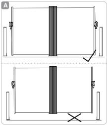
Please note: Please remember that the support post 5 must be mounted in a solid underground (wood, stone). Otherwise the support post 5 will not provide a firm support.
