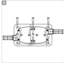
Now insert the dowels 9 into the drill holes (see fig. C).
